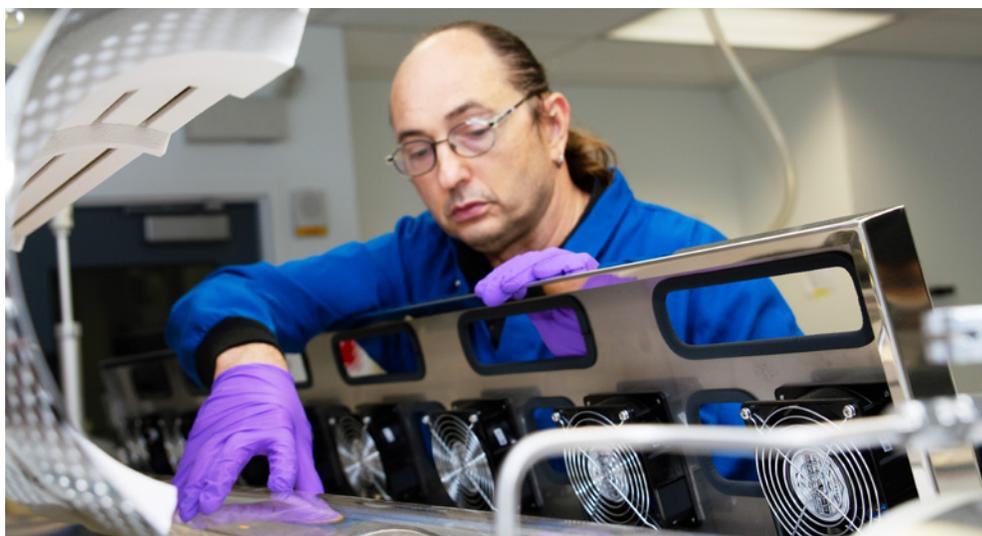
Automated PVD 4-inch sublimator with 7-zone heating system capable of attaining 10<sup>-7</sup> torr.
